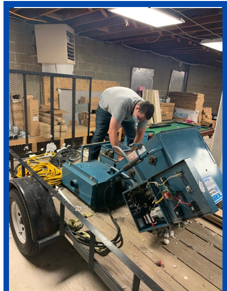
Pictured is Retrofit Installer Terry Moore performing maintenance on the insulation blower.
